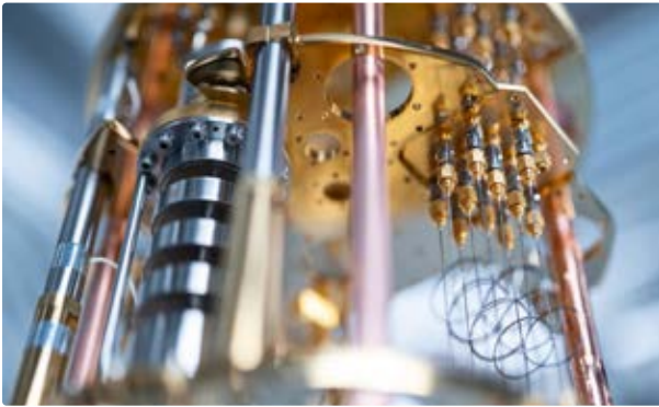
A cryostat to cool down quantum devices to cryogenic temperatures as low as 40 millikelvin. © MQV | Mikka Stampa
